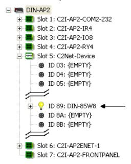
• Additional DIN-8SW8 devices are assigned different Net ID numbers as they are added.
